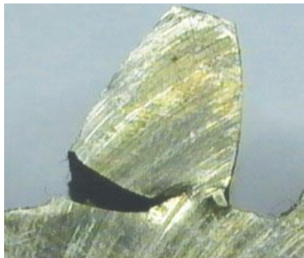
Tooth bending fatigue
