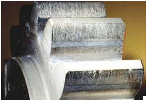
Scuffing (adhesive wear which instantly damages tooth surfaces in relative motion)
