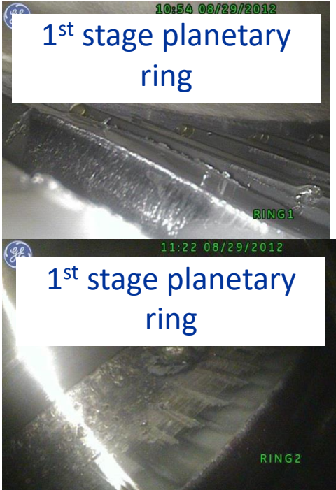
Micropitting (surface failure due to use of surface hardened gears, small craters)
