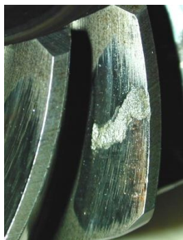
Tooth bending fatigue
