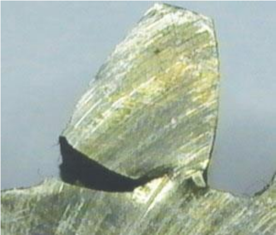
Bending fatigue (due to cyclic bending stress at tooth root)
